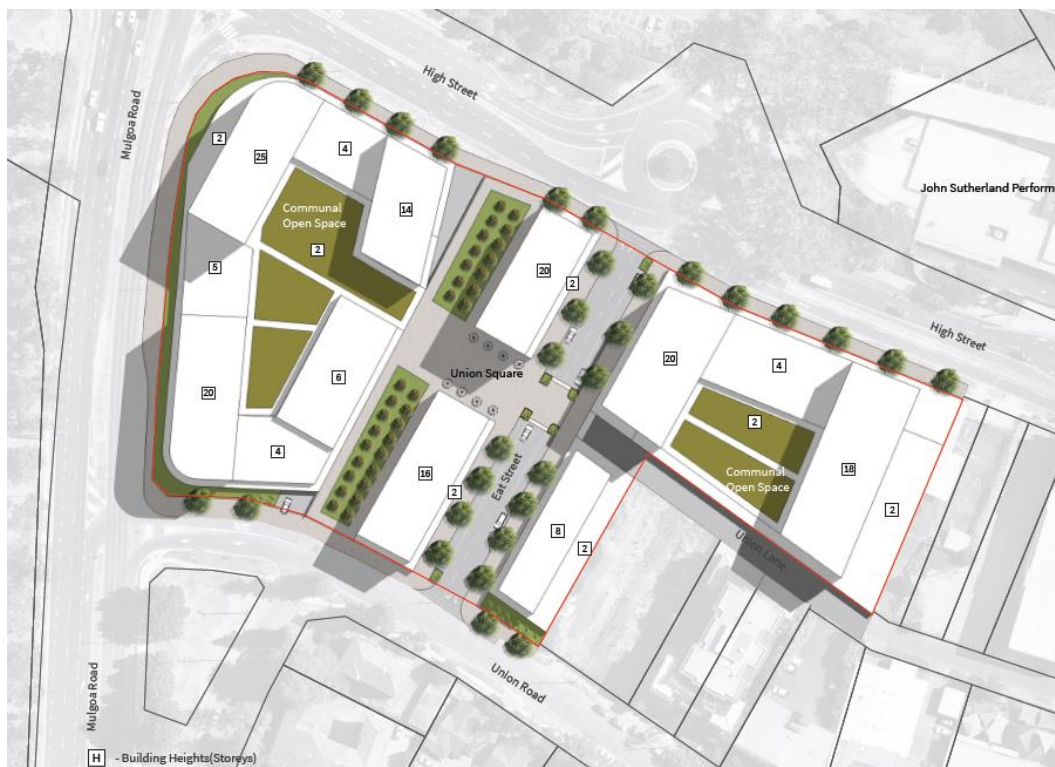
Figure 1 – Site location and proposed built form controls
